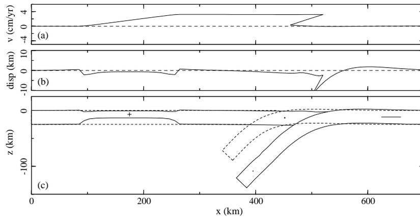
**Figure 8.** Model 11. Subduction zone roll-back in a land-locked basin setting. The side boundaries of the surface plates are fixed laterally. Viscosity of the weak zone in the overriding plate is  $5 \times 10^{21}$  Pa s and  $v_{\text{retr}} = 2$  cm yr $^{-1}$ . Results are shown after 80 km of convergence (after 2.6 Myr). Panels as in Fig. 6.
