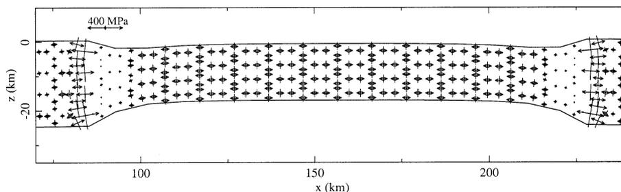
**Figure 9.** Deviatoric stresses in the back-arc region for subduction zone roll-back of model 11 (Fig. 8) after 1.5 Myr.
