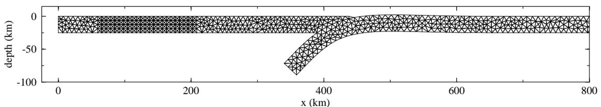
**Figure 1.** Finite element grid. The subducting plate initially extends to 1226 km in the horizontal direction and is not completely shown here. Discretization in the subducting plate is slightly coarser towards the right edge.
